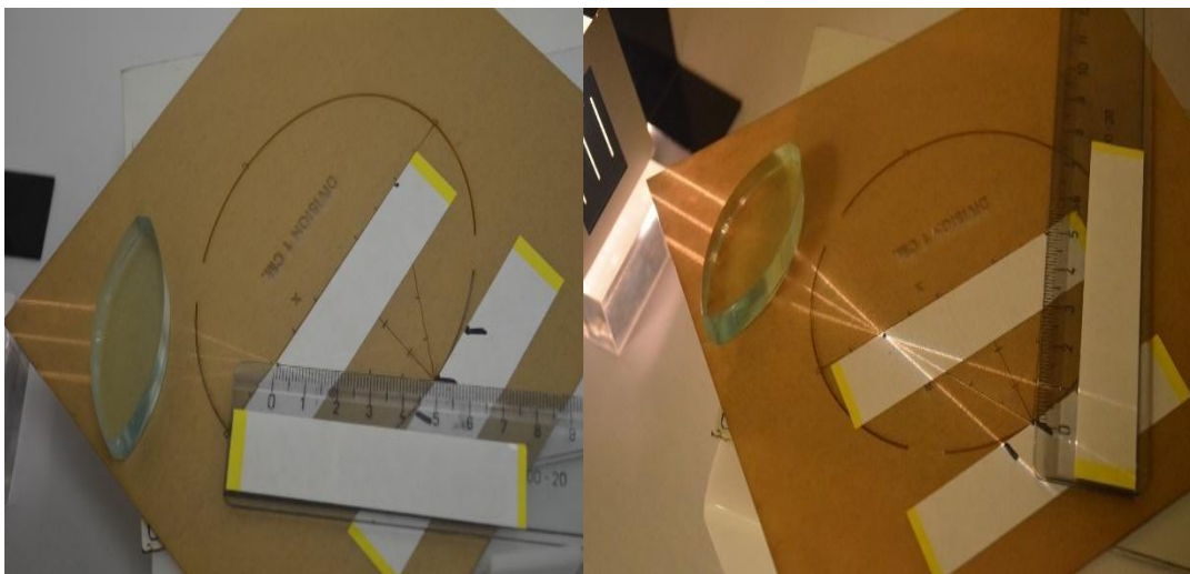
Figure 13: Measurement of a beam from the focus to the vertex of the smaller semi-axis.
