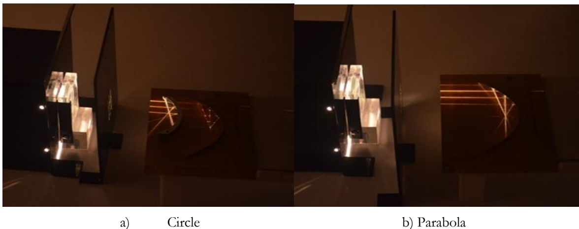
Figure 17: Images of the circle and parabola reflecting beams striking the surface.
