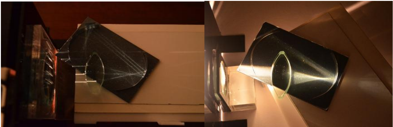
Figure 16: Ellipse projecting parallels beams.
